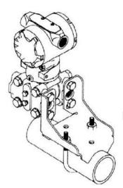
Pipe mounted bent bracket
