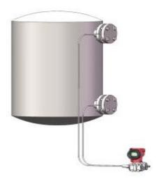
Tank Liquid Level Measurement
